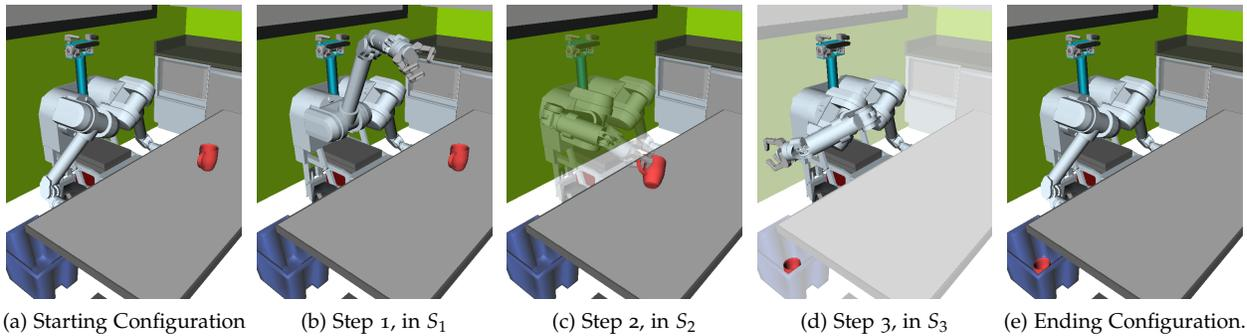
Figure 2.14: A home robot performing a three-step manipulation task. It must move from its home configuration to grasp the cup, transfer it to a drop location above the bin, and return home. Experimental results for the Multi-Set PRM are shown in Table 2.2
