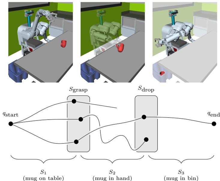
Figure 1.4: Manipulation sub-problems within incongruous free subsets of configuration space. HERB plans for a simple manipulation task to grasp, transfer, and drop a mug from a table into a bin before returning to an end configuration. Each sub-problem requires a path in a distinct free subset of configuration space.
