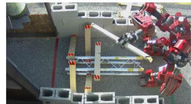
(b) The CHIMP disaster response robot clears debris from a blocked doorway.
