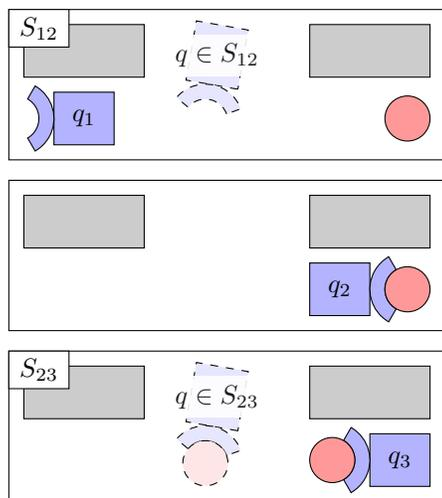
(d) A forklift in a parking lot ( $q_1$ ) must retrieve an object ( $q_2$ ) and reverse park ( $q_3$ ). This two-part problem requires plans in distinct collision-free  $\mathcal{C}$ -subsets  $S_{12}$  and  $S_{23}$ .
